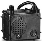
Little Giant makes two pumps that have worked well. The first is one of their smaller and durable pumps - the Model P-AAA. It has an oil-filled motor and pumps at 2 gallons per minute. It is excellent for 4-5 gallon buckets and provides a constant agitation when the discharge fitting is near the bottom and pointed to the side.
