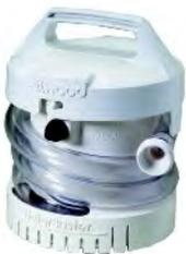
The Attwood WaterBuster is a portable pump that runs on 3 'D' Cell batteries. It pumps for 5 continuous hours at a flow rate of 200 gallons per hour (3.33 gpm) which is fine for agitation purposes. It is available for \$39.95 from West Marine.
