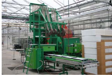
Dickman Farms is currently trialing a new certified sustainable, biodegradable paper with its Ellegaard Ellepot machine for producing its starter plants. Installation of the machine has resulted in the use of less growing media and shorter crop times.
